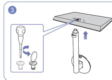
Unfasten the connecting screw at the bottom of the stand base, and then remove the stand neck from the stand base by pulling it in the arrow direction, as shown in the figure.
