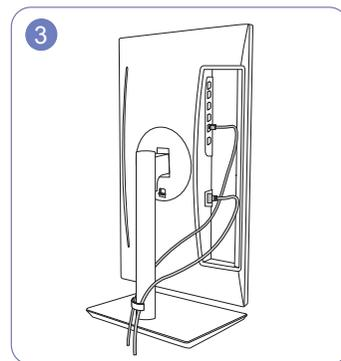
Connect the cables to their correct ports, and then arrange each of the two cables through either side of the COVER-STAND CABLE, as shown in the figure.
