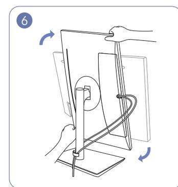
Rotate the machine to the horizontal position.
