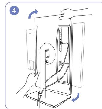
Rotate the machine to the horizontal position.
