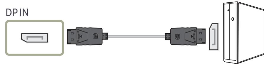
— A DP cable shorter under 1.5 m in length is recommended. Using a cable longer than 1.5 m can affect the picture quality.
